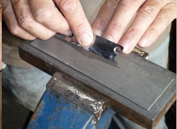
2. Restore bevel by rubbing on the sharpening stone, stoking with a carbide file or...
