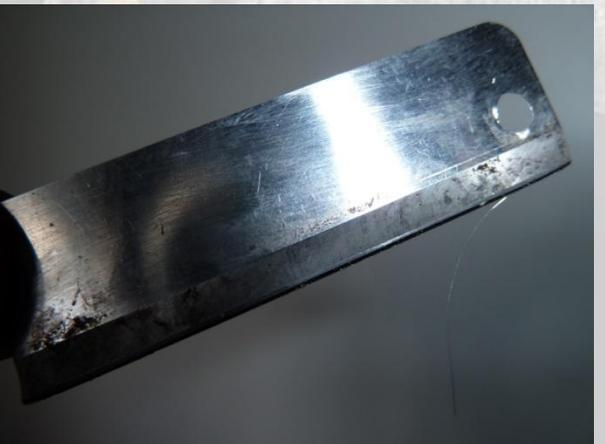
6. Finished tip bevel should be about 1mm. When necessary hone the secondary bevel back to maintain the shape in the same way.
