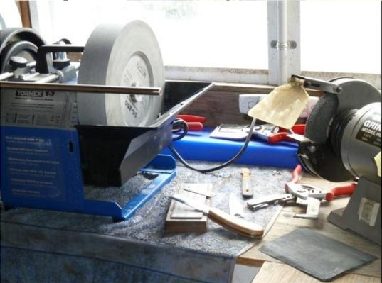
5. Alternatively, use a powered wet grinding stone and finish on a burnishing wheel or leather strop.
