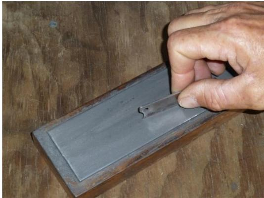
1. Blades have 2mm of tip wear available. If damaged, rub the blade tip and sides on a flat wet sharpening stone.
