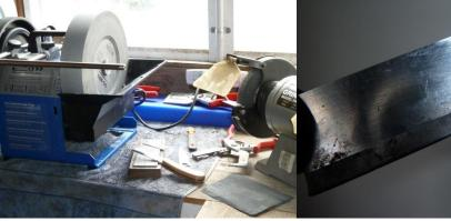
5. Alternatively, use a powered wet grinding stone and finish on a burnishing wheel or leather strop.
