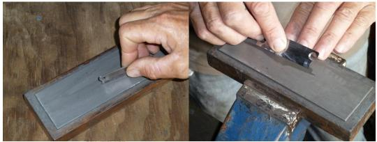
1. Blades have 2mm of tip wear available. If damaged, rub the blade tip and sides on a flat wet sharpening stone.
